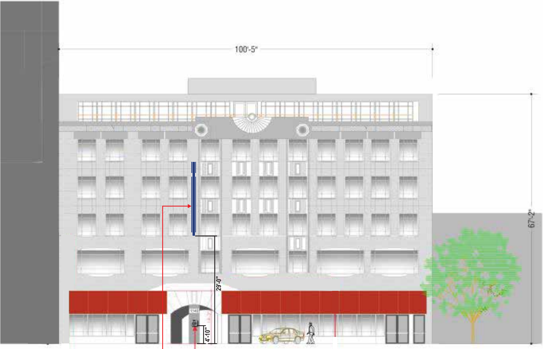
PROPOSED SOUTH ELEVATION SCALE: 1/16"=1'-0"
