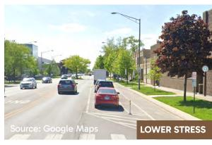
The images above show Madison Street before and after corridor improvements. To the left, the lack of a bicycle facility, 30 MPH speed limit, and number of travel lanes equated to a high level of traffic stress for people bicycling prior to improvements. To the right is a lower stress facility with fewer travel lanes, a parking protected bike facility, and a lower speed limit.
