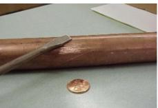
When performing a scratch test, if it turns shiny silver, like the image above, it is likely lead. If the scratched area turns yellow-orange, it is likely copper.
