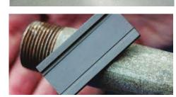
magnet on the pipe. If the magnet sticks to the pipe, it's likely iron and not lead.
